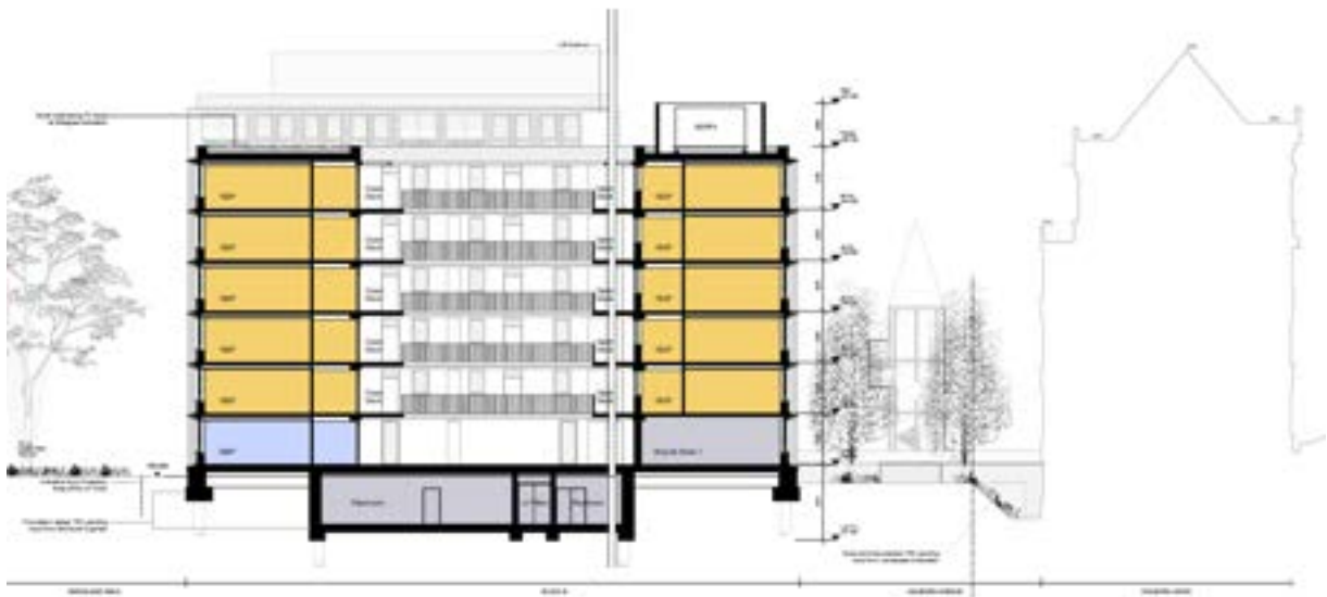
Figure 50: 'Block B Proposed Long Section B0 (East-West)' drawing (AC-NMLA-BB-B0-DR-A-PL200) shows that the roof level plant of Block B (left) would be taller than eaves height of the Main Range (right).
